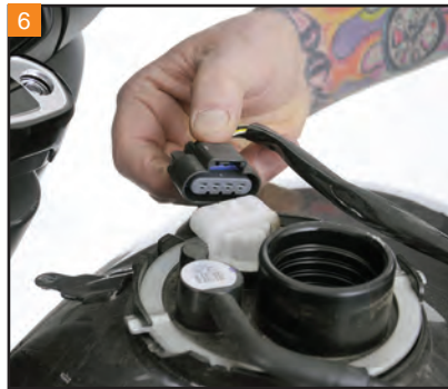
Disconnect the wiring near the filler spout for the fuel pump and fuel level sending unit.
