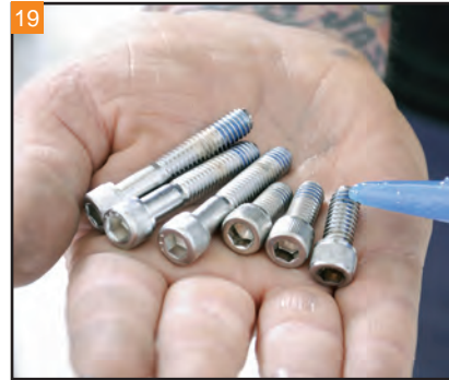
19 Apply blue thread locker to the included hardware from Covington's.
