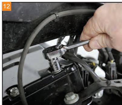
Using a 7/16" socket or wrench, loosen the six bolts holding the stock rocker box top.
