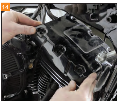
Carefully remove the rocker box top from the right side of the motorcycle.
