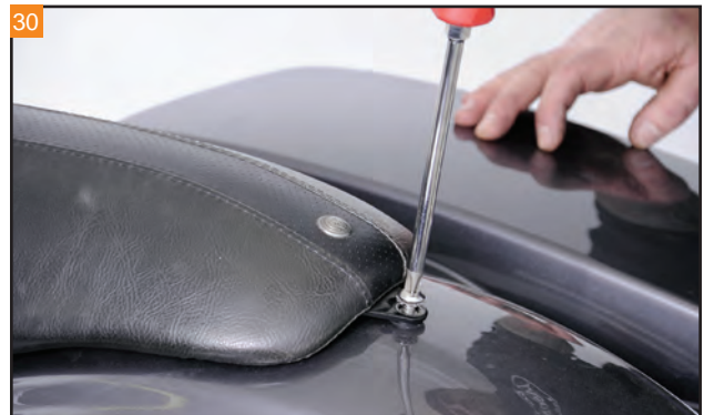
Reinstall the seat back on the motorcycle.
