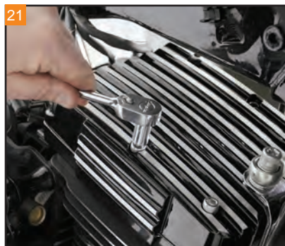
21 Ensure proper placement of the Finned Rocker Top. Begin to tighten the bolts in sequence with a 1/4" Allen.
