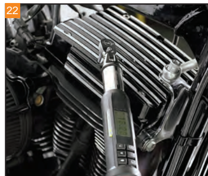
22 Final torque the bolts to 15-18 foot/lbs.
