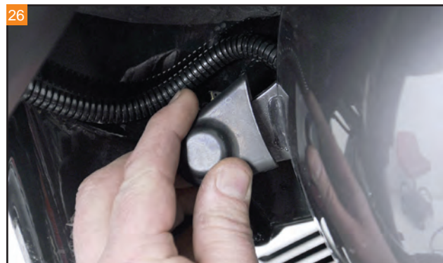
26 Install the rubber covers to the front fuel tank mounting tabs.
