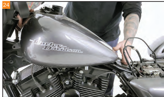
24 Reposition the tank over the backbone of the motorcycle.
