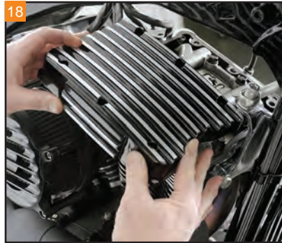
18 Install the Covington's Finned Rocker Top over the lower rocker housing.
