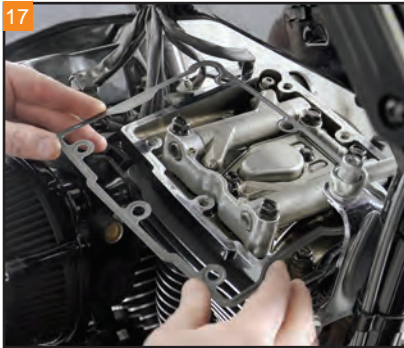
17 Position the new gasket in place. Be sure to orient the gasket correctly.
