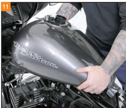
Lift the fuel tank up and off the backbone of the frame.
