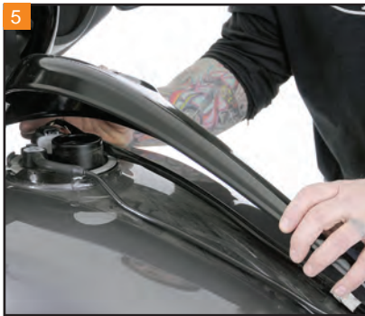
Lift the dash up and off the fuel tank.
