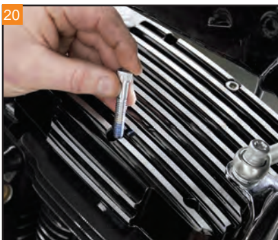
20 Install the six socket head cap screws into the Covington's Rocker Tops. The short bolts go on the left; the long bolts on the right.
