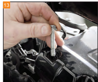
Remove the bolts from the rocker box.
