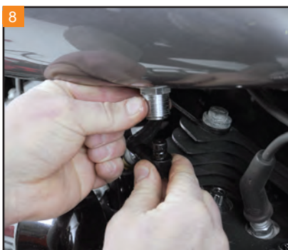
Raise the chrome ring up in order to disconnect the fuel fitting from the tank.
