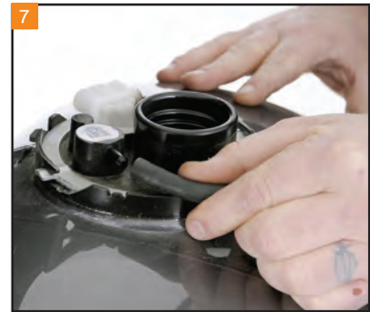
Unplug the vent line from the fitting at the top of the tank.
