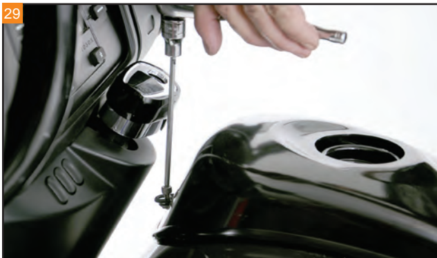
Reinstall the front and rear dash mounting bolts. Screw the filler cap back into the spout.
