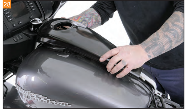
After plugging in the wiring and vent line to the top of the fuel tank, position the dash.
