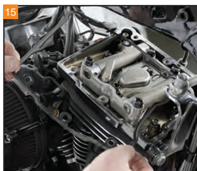
Be sure to remove the stock gasket.
