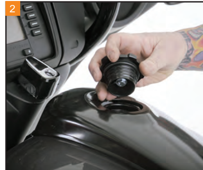
2 To remove the dash from the fuel tank, start by removing the fuel filler cap.
