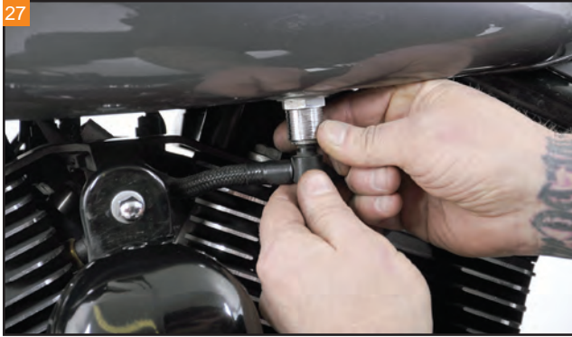
Reconnect the fuel fitting on the left side of the tank.
