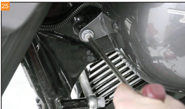
25 Apply blue thread locker to the fuel tank mounting bolts and install. Final torque of 15-20 foot/lbs.
