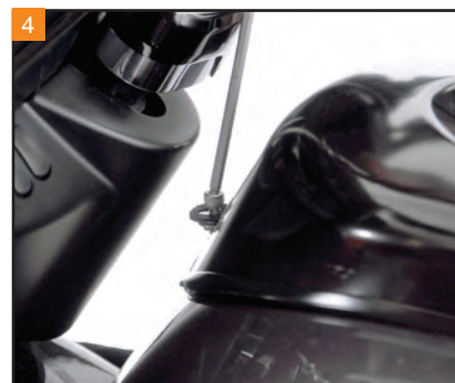
4 With a 5/32" Allen, remove the front dash-mounting bolt.
