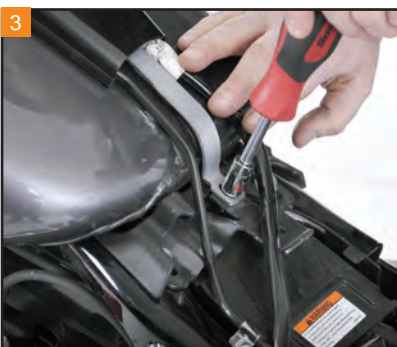
3 Use a 3/8" socket to remove the rear dash-mounting bolt.
