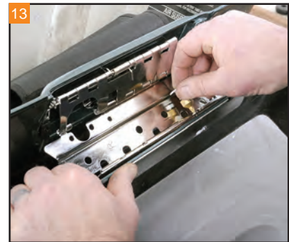
13 Start the screws through the latch and lid, then into the backing plate. It is best to get all five screws started before tightening any of them.
