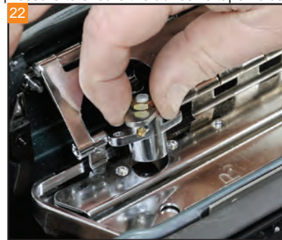
Position the lock assembly in the opening in the latch, aligning the holes in the lock with the threaded holes in the latch cover.
