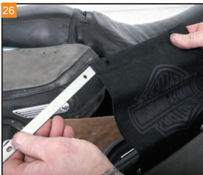
Slide the metal bar through the end of the tether strap, aligning the holes in the strap with the holes in the bar.
