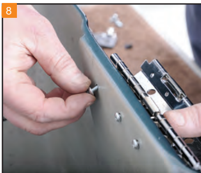
8 Leaving the two inner bolts loose, it is best to start the two outer bolts for proper alignment of the latch.
