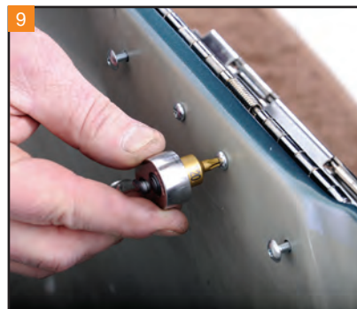
9 Use a T20 Torx to tighten the two inboard bolts.
