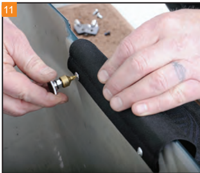
11 Position the tether strap with metal insert and reinstall the two outboard bolts.
