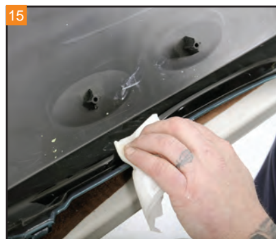
15 Thoroughly clean the gasket channel inside the saddlebag lid with rubbing alcohol.
