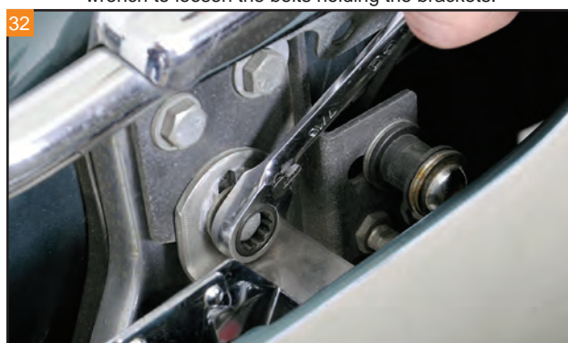
Retighten the bolts holding the brackets in place.
