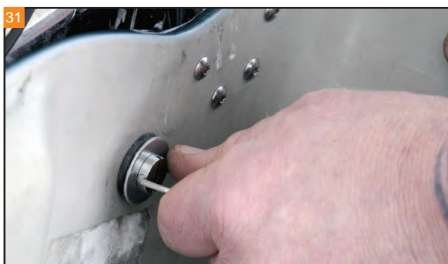
Ensure good engagement of the bail pin in the receptacle.
