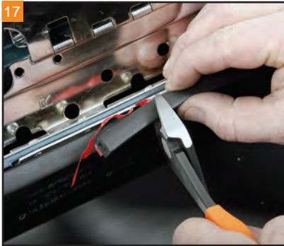
Trim any excess gasket material with side cutters.
