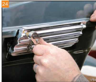
Install the included chrome bolts from Covington's from the outside of the latch cover.
