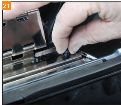
From the inside, start the #8 bolt through the latch into the threaded hold of the latch cover. Leave the bolt loose for now, until all the latch cover hardware and lock is installed.
