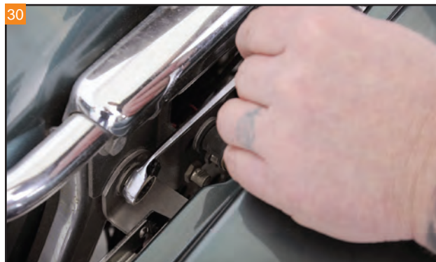
It may be necessary to loosen the brackets for best alignment with the new bags. Use a 7/16" wrench to loosen the bolts holding the brackets.
