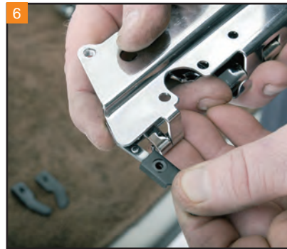
6 Slide the rubber bars over the tabs of the saddlebag latches. The rubber bars are side specific.
