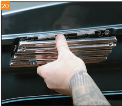
Position the Covington's Finned Latch Cover in place over the saddlebag latch.
