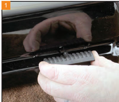
Insert the support cushions, two per bag, into the channel in the bottom of the saddlebags. A small amount of spray lubricant will help to get the tip of the cushion through the hole in the saddlebag.
