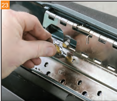
Use blue thread locker on the hardware. Tighten the lock mounting hardware with a Torx driver.
