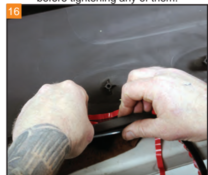
16 Remove the plastic covering from the adhesive on the weather gasket. Install the gasket in the channel of the lid, applying pressure to ensure the adhesive tape holds.
