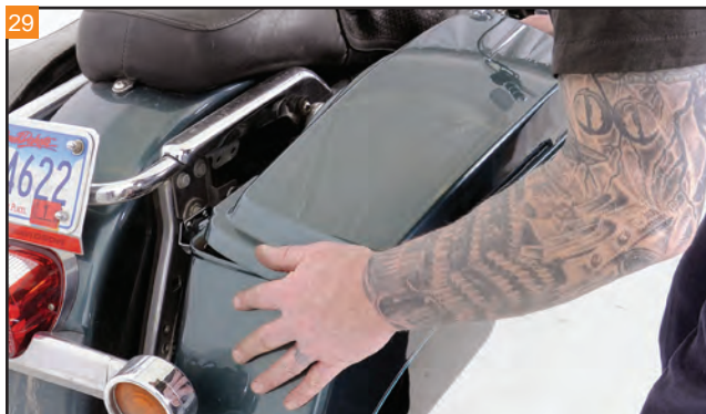
Position the assembled hard bag on the saddlebag support bar.
