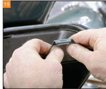
Remove the protective plastic from the adhesive tape on the back of the wear plate. Position the wear plate on the lid, applying pressure to ensure the adhesive tape holds.
