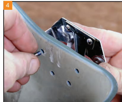
Start the four bolts for the mounting bracket by hand.
