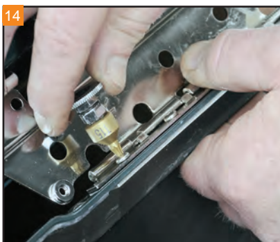
14 With all five screws started, use a T15 Torx to tighten them down.
