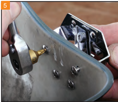
5 Final tighten the hardware with a T15 Torx driver.
