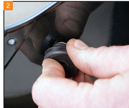
Install the bail pin grommets in the holes on the inner side of the bags. The thicker portion of the grommet is on the outside of the bag.
