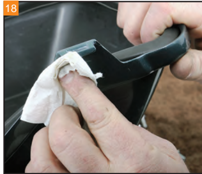
Clean the area of the lid for the wear plates thoroughly with rubbing alcohol.
