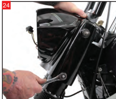
Reinstall the nacelle. Leave the acorn nuts loose for now.
