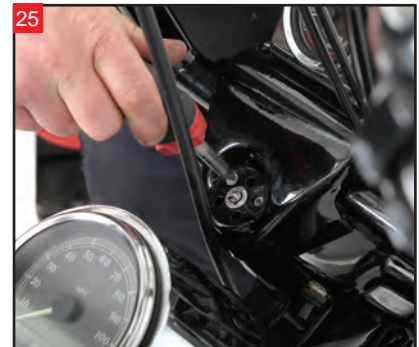
Install the handlebar riser cover. Use a Phillips screwdriver to tighten the two screws at the fork lock. Push the plastic cover over the fork lock.
