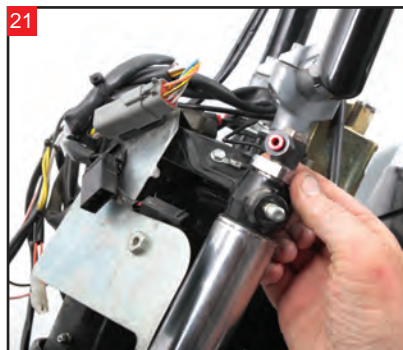
Install the fork cap bolt into the fork cap. Final torque to 11-22 foot/lbs.
