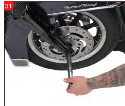
Reinstall the front wheel, spacers, and front axle.
