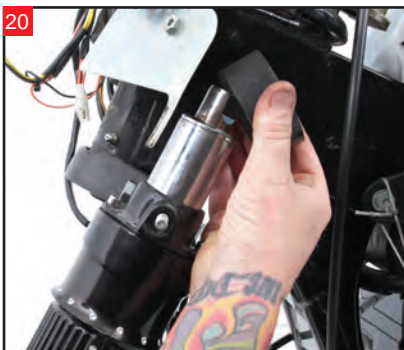
Bring the fork leg back into position. Install the fork stop bumper over the fork leg before inserting the leg into the top triple tree.
