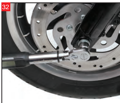
Holding the front axle in place, final torque the front axle nut to 50-55 foot/lbs.
