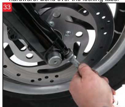
Use a 1/2" wrench to tighten the axle clamp nuts. Final torque to 9-13 foot/lbs.
