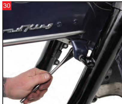
Apply blue thread locker to the front fender bolts. Position the front fender between the fork sliders. Use a 1/2" socket to tighten the hardware. Bend over the locking tabs.
