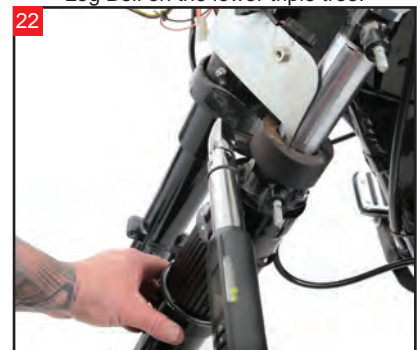
Apply blue thread locker to the pinch bolt. Final torque the pinch bolt to 40 foot/lbs.
