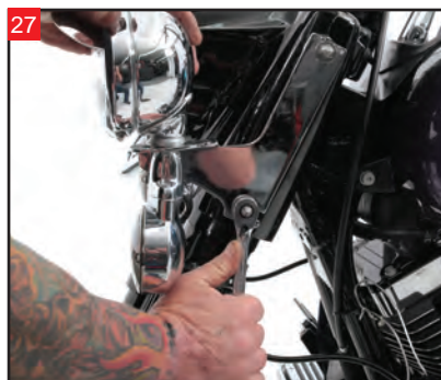
Reinstall the passing lamp assembly. Plug in the wiring. Final tighten the acorn nuts with a 1/2" wrench.
