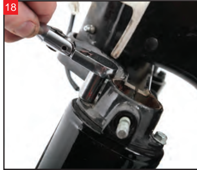
Use a 3/8" socket to loosen the bolts holding the stock upper fork slider cover to the lower triple tree.
