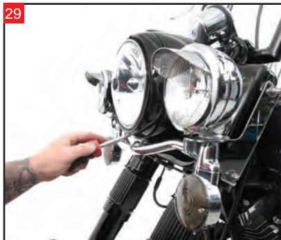
Reinstall the trim ring with single screw at the 6 o'clock position.
