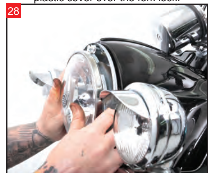
Plug in the connector to the back of the headlamp. Position the headlamp assembly in the nacelle. Install the screws using a Phillips screwdriver.
