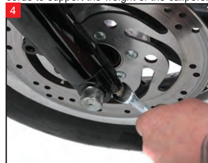
With a 1/2" wrench, loosen the axle clamp hardware on the right fork slider.
