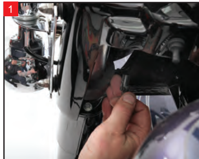
From the back of the nacelle, disconnect the wiring for the front fender tip light.
