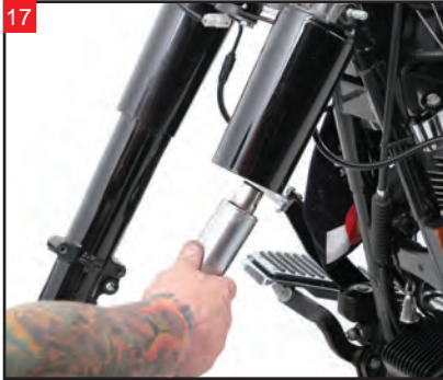
Slide the fork leg out from the triple trees.
