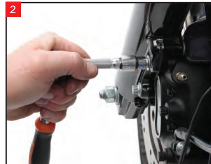
Use a 10mm 12-point socket to remove the caliper mounting hardware. Remove the calipers from the rotors. Use bungee cords to support the weight of the calipers.
