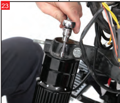
Repeat the process for the second Covington Fork Leg Bell.
