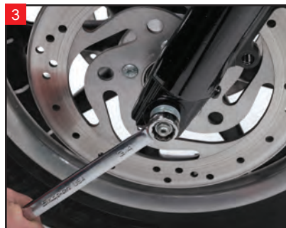
Support the frame with a center jack. Loosen the front axle nut using a 3/4" wrench.
