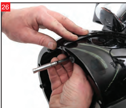
Use a 5/16" socket to tighten the nut holding the top cover to the nacelle.
