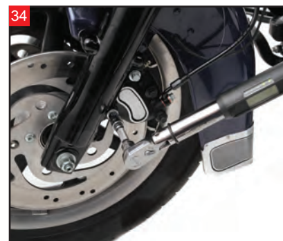
Reinstall the front brake calipers. Use blue thread locker on the bolts. Final torque the hardware to 28-38 foot/lbs.
