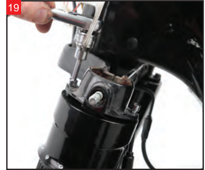
Apply blue thread locker to the supplied hardware. Use a 3/16" Allen to install the Covingtons Fork Leg Bell on the lower triple tree.
