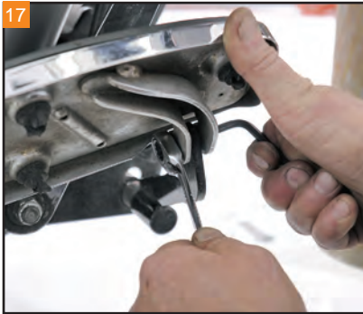
17 Loosen the right side floorboard hardware with a 3/16" Allen and 7/16" wrench.
