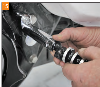
Install the Covington's Passenger Peg with spring washer into the peg mount.
