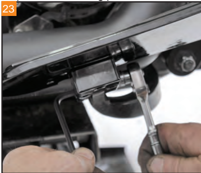
23 Install the floorboard using the stock hardware.
