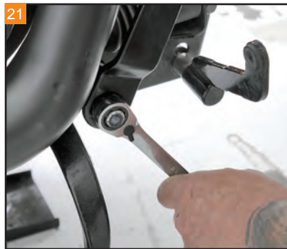
21 Use a 5/8" wrench to tighten the nylock nut onto the end of the pivot shaft, with washer.
