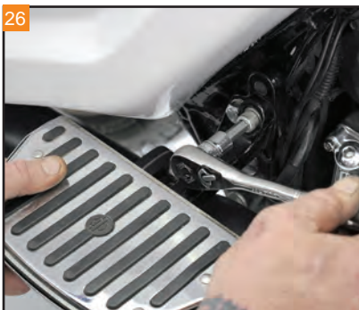
26 Remove the bolt holding the right side passenger floorboard mount to the frame with a 5/16" Allen wrench.
