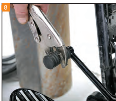
Use locking pliers to remove the stock rubber shift peg from the shift arm.
