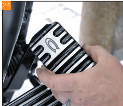
24 Place the Covington's Fined Brake Pedal over pedestal of the brake arm.
