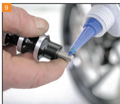
Apply blue thread locker to the included hardware for the Covington's shift pegs.
