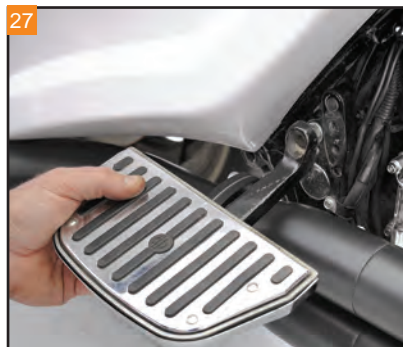
27 Remove the passenger floorboard and mounting bracket as an assembly.
