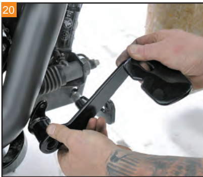
20 Slide the new black brake arm over the pivot shaft, ensuring the arm engages the actuator of the master cylinder. Install the pivot and retaining pins with washer.
