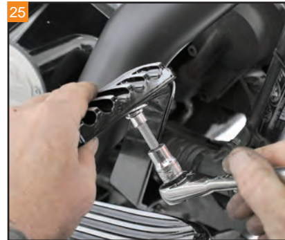
25 Apply blue thread locker to the included hardware for the brake pedal. Tighten with a 1/4" Allen wrench.
