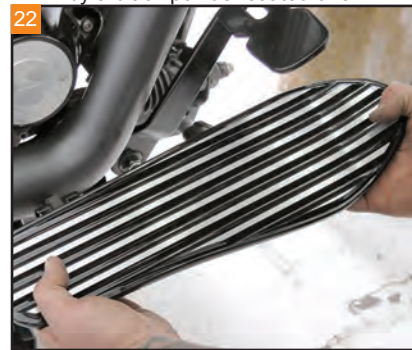
22 Position the right side Fined Floorboard over the mounting brackets.
