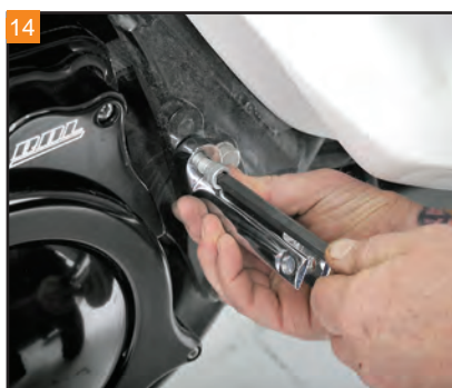
Apply blue thread locker to the stock bolt. Install the Drag Specialties passenger peg mount in the stock location of the floorboard bracket.
