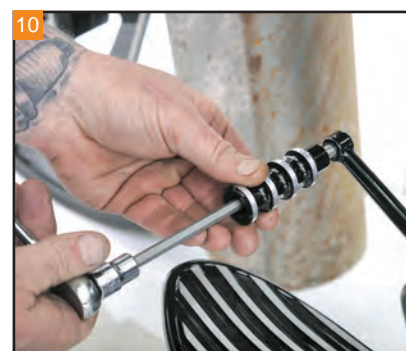
Use a long 1/4" Allen to tighten the bolt holding the shift peg to the shift arm.
