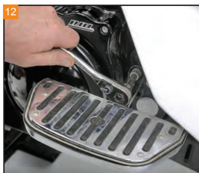
Remove the bolt holding the stock passenger floorboard bracket with a 5/16" Allen.
