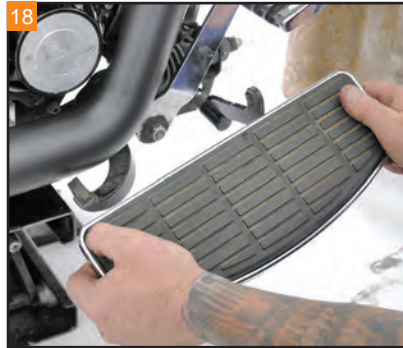
18 Remove the floorboard from the mounting brackets.
