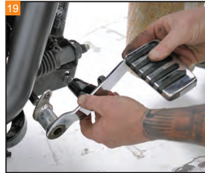
19 In order to match the Covington's Fined Black Brake Pedal, the stock chrome brake arm is going to be replaced by a black powder coated one.
