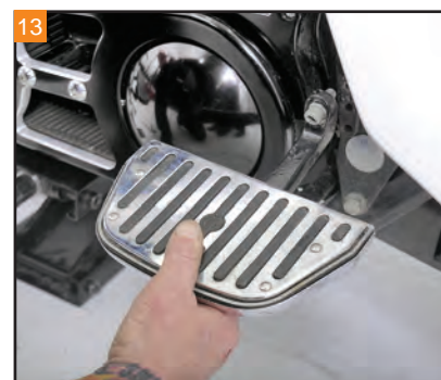
The passenger floorboard and mounting bracket can be removed as an assembly.
