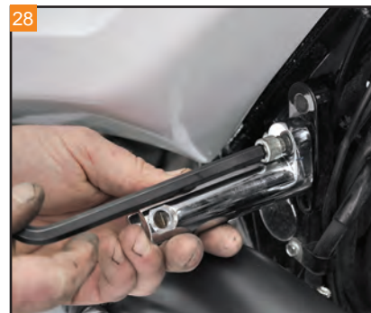
28 Install the Drag Specialties Passenger Peg Mount using the stock hardware. Use blue thread locker on the bolt.
