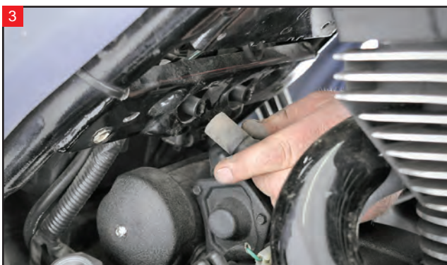
Unplug the spark plug wires from the coil. The right side post is for the rear head, and the left side coil post is for the front.
