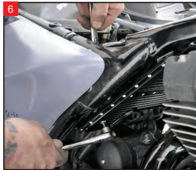
Using a 5/32" Allen and 7/16" wrench, tighten the hardware down uniformly.
