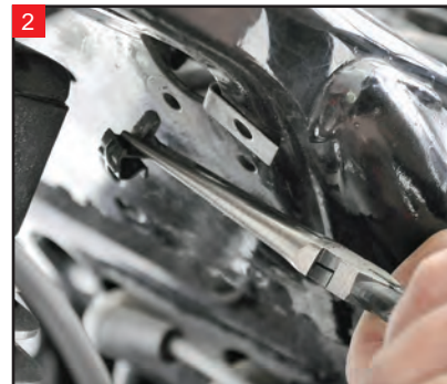
Use a set of needle nose pliers to remove the zip tie from the frame for the spark plug wire.
