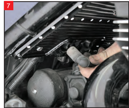
Reinstall the spark plug wires back onto the coil. Ensure the front and rear spark plug wires are on the correct post of the coil.
