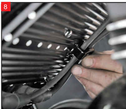
Capture the spark plug wires with the included bracket from Covingtons. The bracket will replace the use of zip ties to hold the spark plug wires in position.
