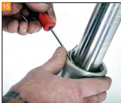
15 Move the fork slider all the way down the fork leg. With a small flathead screwdriver, remove the retaining ring from above the fork seal.
