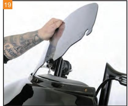
Lift the windshield up and out from between the inner and outer fairing.
