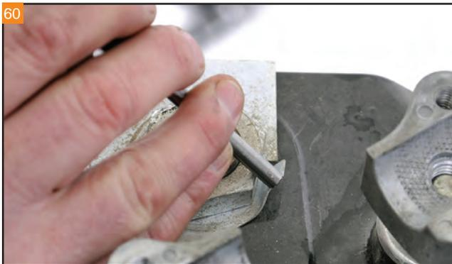
Before removing the neck stem nut, use a punch and hammer to bend the locking tab down.
