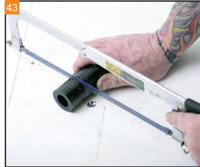
Use a hacksaw to cut the travel limiter to length. Ensure the cut is as straight as possible.
