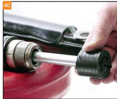
Position the limiter over the bottom cup of the fork leg.
