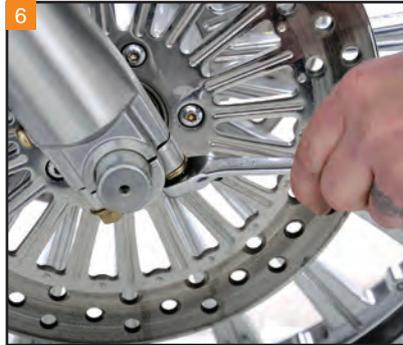
6 With a 1/2" wrench, loosen the two nuts holding the axle clamp.
