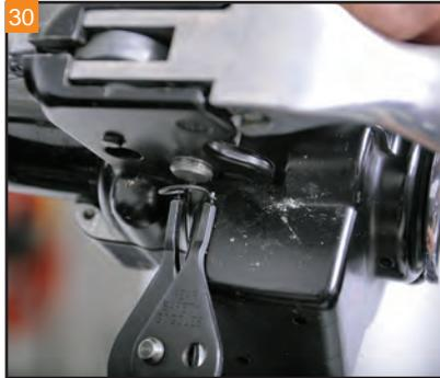
Use retaining ring pliers to remove the retaining ring from the clutch lever pivot pin in the left side hand controls. Lift the pivot pin up and out of the clutch perch.
