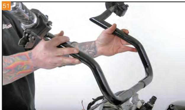
Lift the handlebars off the risers as an assembly.
