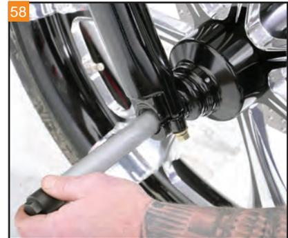
58 Slide the axle in from the right side, through the fork slider, wheel spacers, and wheel hub.
