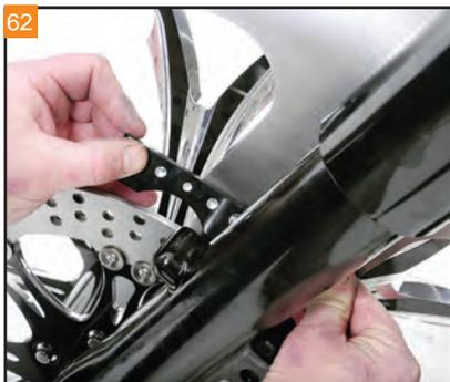
62 Reinstall the front fender with spacers and hardware.
