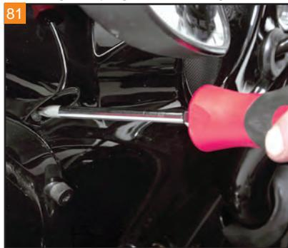
81 With a T27 Torx, install the four bolts holding the outer fairing to the inner.
