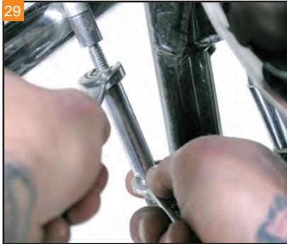
Loosen the clutch cable adjuster in order to introduce slack in the clutch cable.
