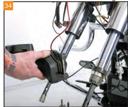
The brake line and calipers can be removed as an assembly from the motorcycle.
