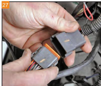
Unplug the wiring from the motorcycle main wiring harness to the fairing interconnect harness.
