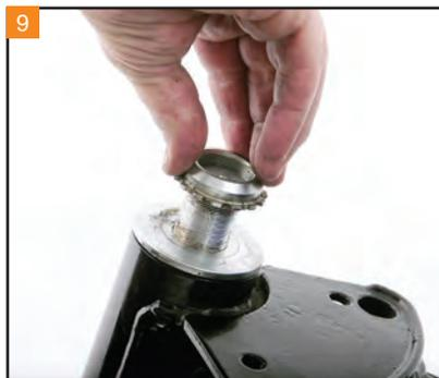
Position the neck stem in the frame neck. Install the dust cover and top spanner nut.
