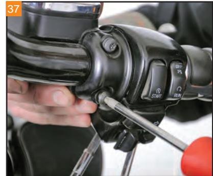
Remove the bolts holding the master cylinder assembly to the handlebars with a T27 Torx.
