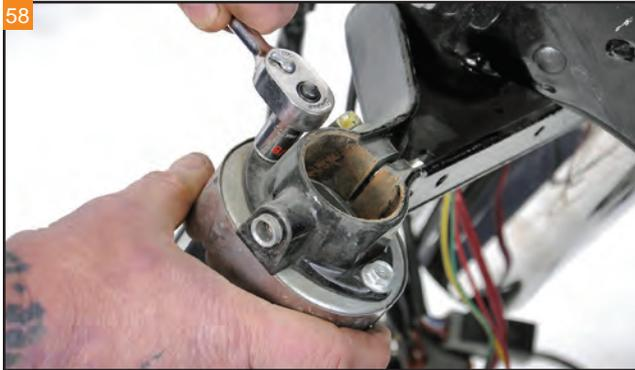
Using a 3/8" socket, remove the two bolts holding the upper fork slider cover to the lower triple tree.
