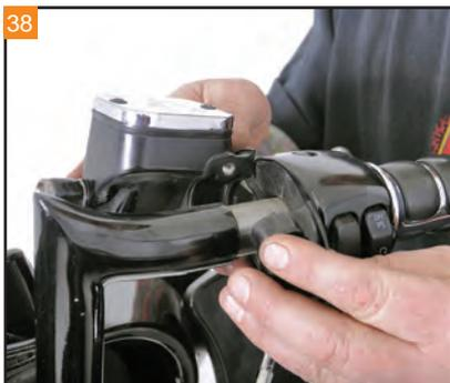
The front master cylinder can be removed from the handlebars.
