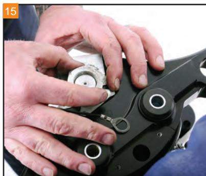
Reinstall the top triple tree with stem nut and locking plate.
