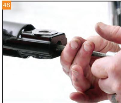
Install the damper bolt with new crush washer. Tighten with a 6mm Allen. Final torque to 132-216 inch/lbs.
