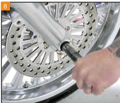
8 Maintain control of the wheel and spacers when removing the axle.
