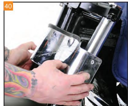
40 Temporarily install the lower outer chrome fairing skirt over the triple trees. Use the stock hardware to hold it in place.
