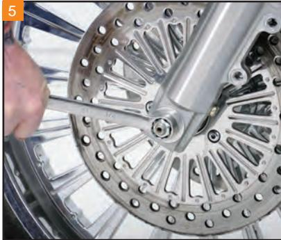
5 Use a 3/4" wrench to loosen the front axle nut on the left side.
