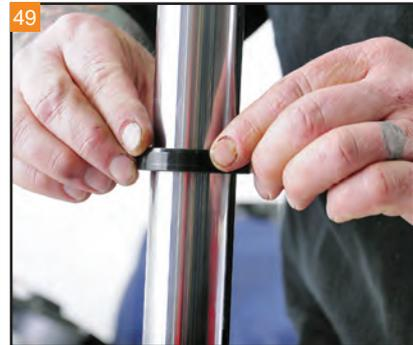
Use a **new** 41mm fork seal from the James Gaskets Kit, with retaining ring.
