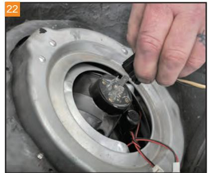
Squeeze the two sides of the connector in order to release it from the headlight.
