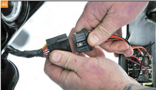
46 Unplug the wiring for the switches in the lower inner fairing.
