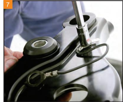
Using a 5/16" socket, install the ground wire and bolt in the threaded hole in the Ness KO Trees.
