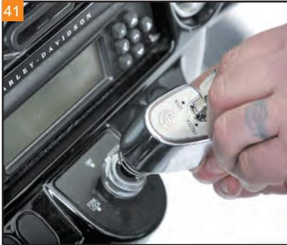
41 Insert the key in the ignition switch. Mash the detent on the bottom of the switch while rotating the key counter-clockwise past unlock. Lift the ignition switch out of the post.
