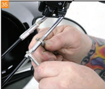
Loosen the adjusters in the throttle and idle cables in order to introduce slack in the cables.
