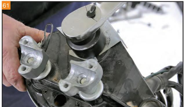
With a 1 1/2" socket, loosen the neck stem nut.
