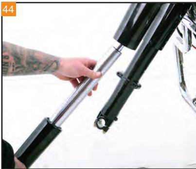
Remove and disassemble the fork legs from the fork sliders.
