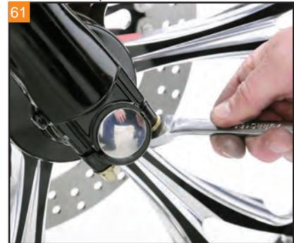
61 Install the end cap in the right side fork slider. Tighten the hardware with a 1/2" wrench. Final torque is 5-11 foot/lbs.
