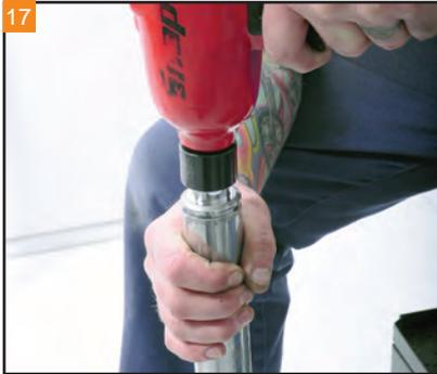
17 Remove the fork leg top cap with specialty socket and impact wrench. Use caution as the internal spring causes the top cap to be under pressure. Apply slight pressure down when removing.
