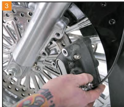
3 Slide the caliper off the rotor.
