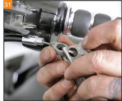
Remove the clutch lever from the perch in order to remove the cable from the lever. Route the clutch cable out and clear from the fairing.
