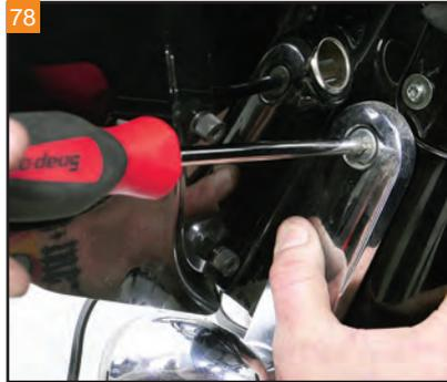
78 Reinstall the front turn signals, using a T40 Torx to tighten the hardware. Don't forget to plug in the turn signals.
