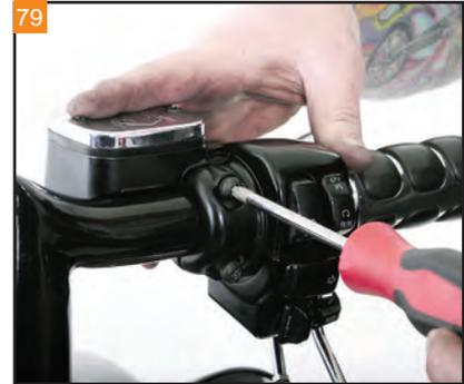
79 Route and reinstall the throttle, idle, and clutch cables. Adjust the clutch and cables as necessary.
