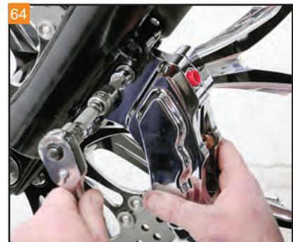
64 Use the included hardware and large spacers to initially mount the caliper.
