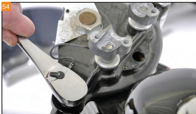
Remove the fork cap nut from the top of the fork leg with the specialty socket.
