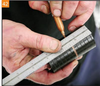
Follow the formula found in the Ness Triple Tree Instructions to determine the length of travel limiter needed. Mark the limiter accordingly.
