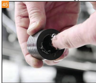
Thoroughly coat the inside of the travel limiter with grease.
