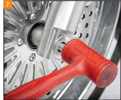
7 Use a center jack to support the frame of the motorcycle, taking the weight off the front end. Gently tap the axle out from the left side of the motorcycle with a rubber mallet.
