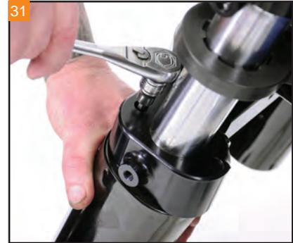
31 Use a 3/16" Allen to tighten the bolts for the upper fork slider covers.
