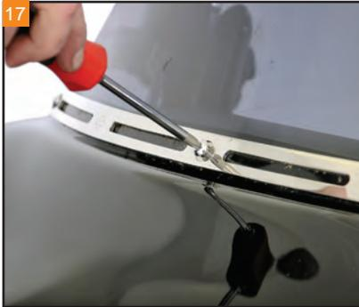
Remove the three windshield bolts with a T27 Torx.
