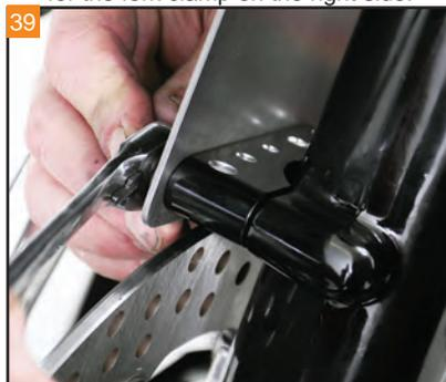
39 Tighten the hardware with a 1/2" wrench.
