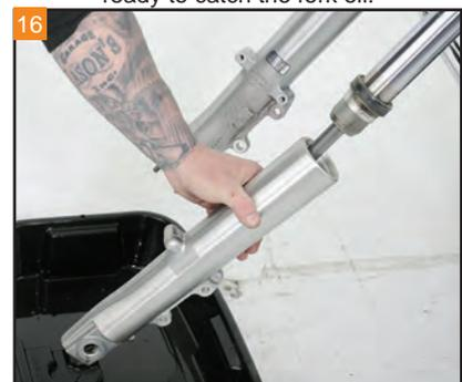
16 In a "slide hammer" motion, remove the fork slider from the fork leg. Repeat the process for the other side.
