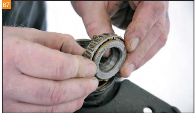
Inspect the top neck bearing, along with the upper and lower neck bearing races for excessive wear and are need of replacing.
