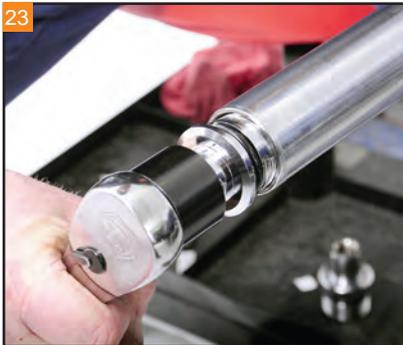
23 Tighten the top cap into the fork leg by hand. A light coat of fork oil on the included O-ring is recommended. Snug, do not final tighten, the top cap at this time.
