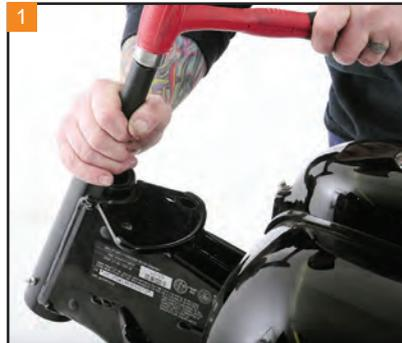
1 Remove the upper and lower bearing races with the removal tool.
