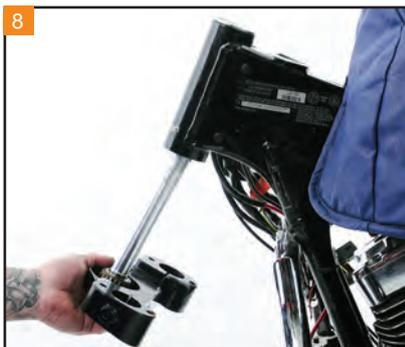
After applying grease to the lower neck bearing, bring the lower triple tree neck stem up through the frame neck.
