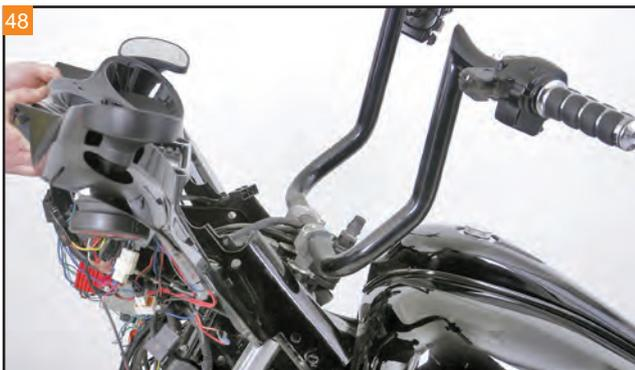
48 Remove the inner fairing by lifting it up and off the triple trees.
