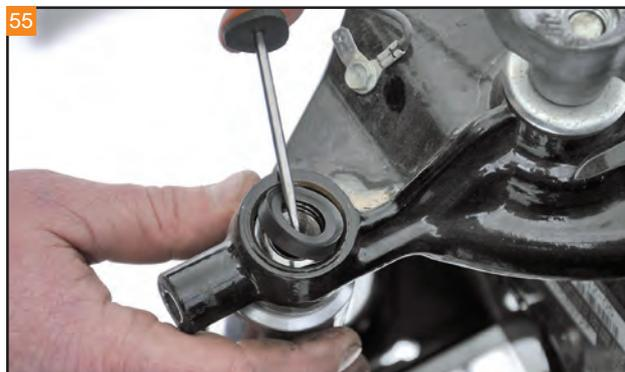
Using a small pick, remove the rubber seal from the top of the fork leg.
