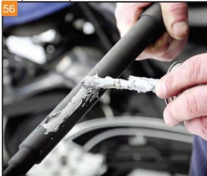
56 Apply a **light** coat of anti-seize lubricant to the Klock Werks' Axle. The threads of the axle are treated with blue thread locker.
