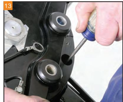
Bring the front end to the left stop, and back approximately a 1/2". Mark a circle on the top plate of the frame with an awl or scribe for a new fork lock hole.
