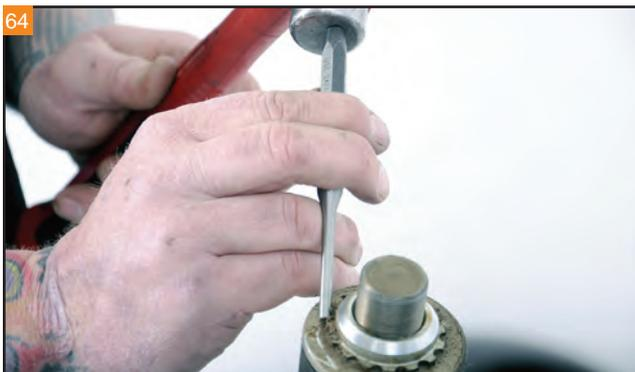
Loosen the spanner nut found underneath the top triple tree. Maintain control of the lower triple tree while loosening the nut.
