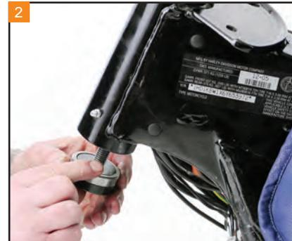
2 Place the new neck bearing races in the installation tool.
