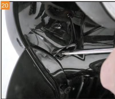
With a T27 Torx, remove the four bolts holding the outer fairing to the inner. Maintain control of the outer fairing while doing so.
