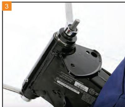
3 Apply a small amount of clean oil to the outside of the bearing races. Install the new neck bearing races into the neck.
