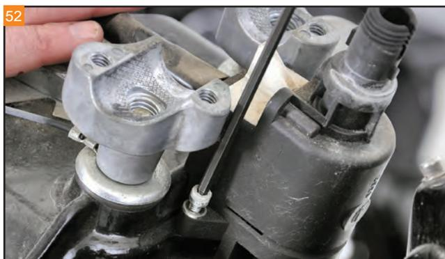
Use a 5/32" Allen to remove the two bolts holding the ignition switch assembly.
