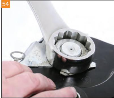
54 Using a 1 1/2" wrench tighten the neck stem top nut. Final torque of 60-80 foot/lbs. Ensure to bend the locking tab. Verify the adjustment of the neck bearings.
