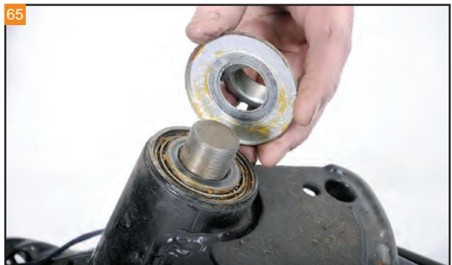
Remove the nut and dust shield from the neck stem.
