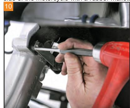
10 Bend the locking tabs down around the fender mounting bolts with a small punch and hammer.
