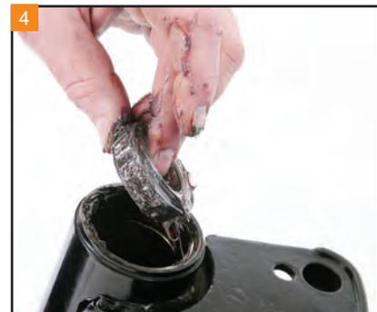
4 After greasing the new upper neck bearing, place it in the upper section of the neck.
