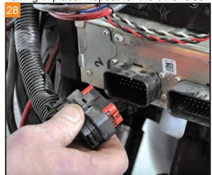
Unplug the radio and wiring coming from the handlebar controls.
