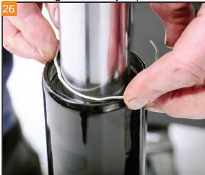
26 Position the **old** seal using the fork seal installer. Reinstall the **old** retaining ring over the seal, in the groove in the fork slider. Repeat the process for the other fork leg.
