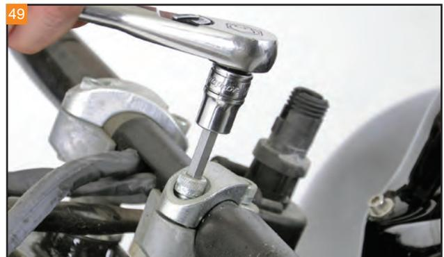
49 Loosen the riser clamp bolts with a 1/4" Allen. Maintain control of the handlebars while doing so.
