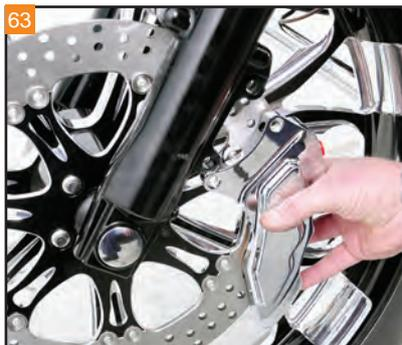
63 Position the HHI caliper over the rotor.
