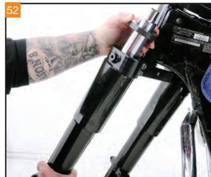
Install the assembled fork legs with rubber stops back into the triple trees.
