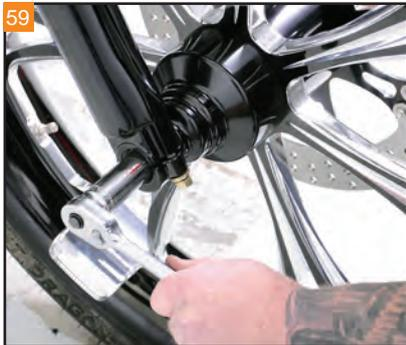
59 Use a 3/4" deep well socket to tighten the axle. Use caution to **not** cross thread the axle in the end cap.
