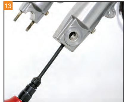
13 Use a 6mm Allen to remove the damper bolts from the bottom of the fork sliders. Have a drain pan ready to catch the fork oil.
