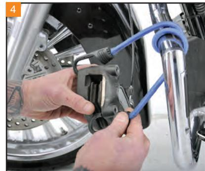
4 Support the weight of the caliper with a bungee cord; do not let it hang from the brake line. Repeat the process for the other front brake caliper.
