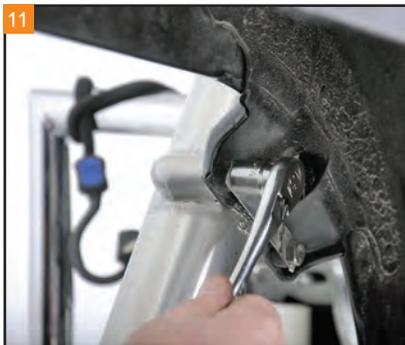
11 With a 1/2" socket, remove the four fender mounting bolts.
