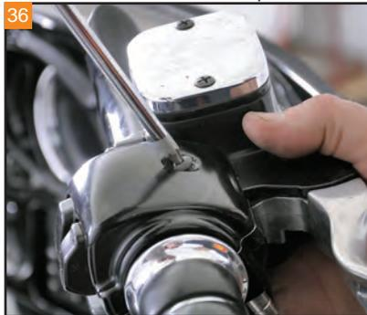
With a T25 Torx, remove the two bolts holding the switch housing together.
