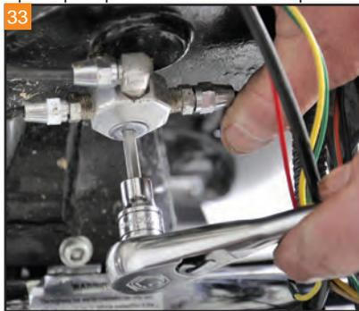
Route the front brake line through the fairing and out. Remove the bolt holding the brake line junction block under the lower triple tree.
