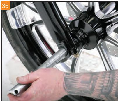
35 Install the stock axle with included spacers from Performance Machine, through the right side fork slider and hub.
