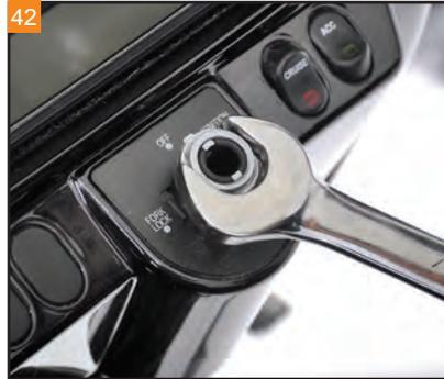
42 Use a 7/8" wrench to remove the plastic nut from the ignition post. Remove the two remaining plastic pieces from the post.
