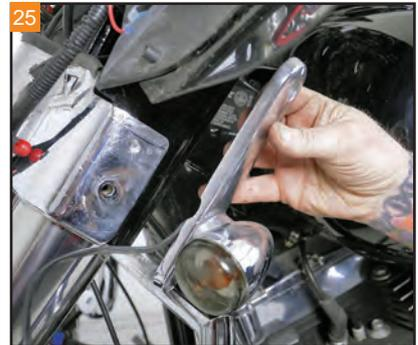
Remove the turn signal assembly from the motorcycle. Reinstall one of the turn signal mounting bolts back into a threaded hole to hold the inner fairing in place. Repeat for the other side.
