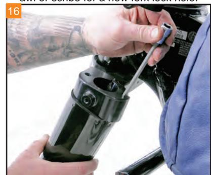
Loosely install the upper fork slider covers with the hardware included with the Ness Trees. Use blue thread locker on the bolts, but do not tighten at this time.
