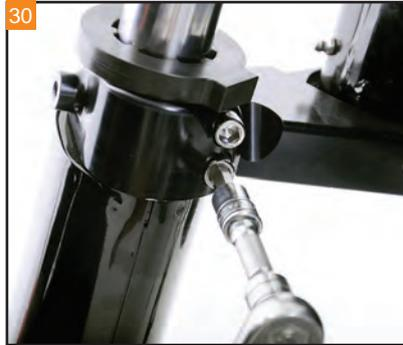
30 Tighten the two pinch bolts in the lower triple tree.
