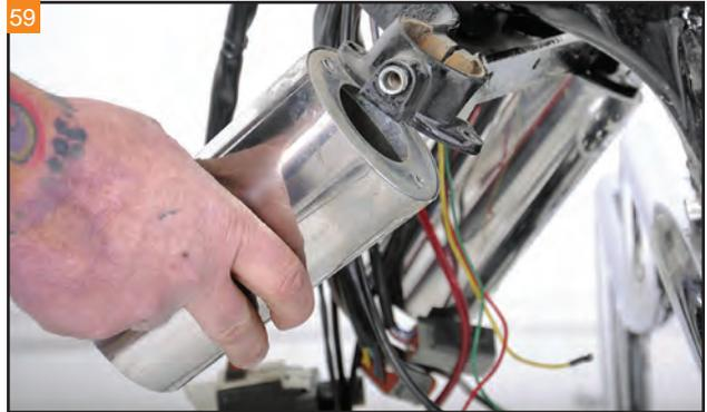
Remove the upper fork slider cover. Repeat the process for the other side.
