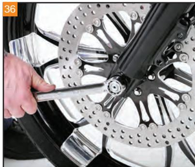
36 Tighten the axle nut with a 15/16" wrench while holding the axle stationary. Use a 1/2" wrench to tighten the hardware for the fork clamp on the right side.
