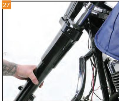
27 Bring the fork leg into position in the triple trees. Do not forget the included new fork stop on the leg.
