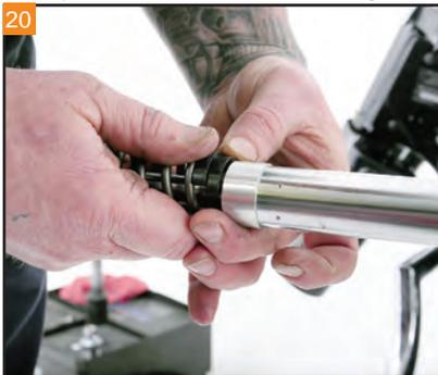
20 Install the two plastic "c" shaped spacers onto the Monotube Assembly.
