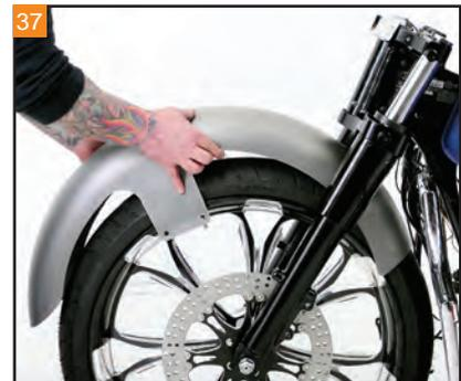
37 Bring the fender into position over the front wheel.
