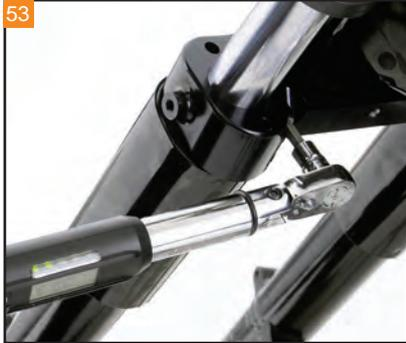
53 After installing the fork cap top nut (final torque of 50-60 foot/lbs.), tighten the two pinch bolts in the lower triple tree. Use blue thread locker on the bolts. Final torque of the pinch bolts is 28-35 foot/lbs.
