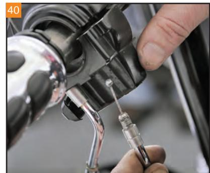
The cable housings can be removed from the switch housings by pulling them straight down. Feed the cables through the inner fairing and clear of the front end.
