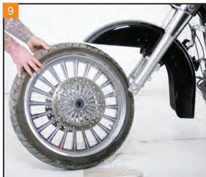
9 Use the center jack to raise the front end enough to remove the front wheel.
