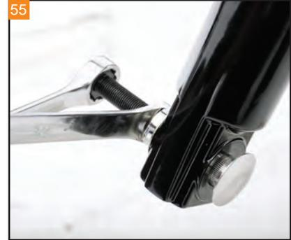
55 Use the included bolt, nut, and washer to install the Klock Werks' splined end cap in the left side fork slider.
