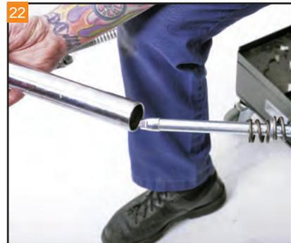
22 Insert the Monotube Assembly into the fork leg.
