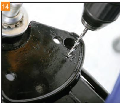
Create a mark with a punch in the center of the circle scribed on the frame plate. Drill a pilot hole first. Continue to enlarge the bit size until a 1/2" hole is made.
