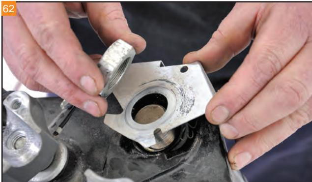
After removing the nut, lift the locking tab plate up and off the neck stem and top triple tree.
