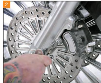
2 With a 10mm 12pt socket, remove the two bolts holding the brake caliper to the fork slider.
