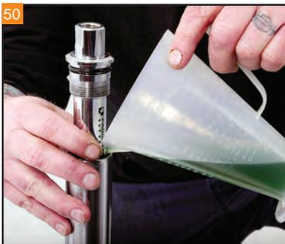
After loosening the fork cap from the fork leg, pour five ounces of 10-weight fork oil into the fork tube.
