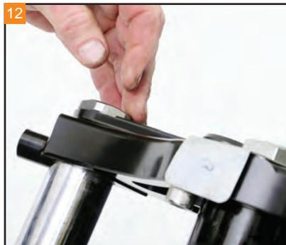
Hold the leg in place with the top fork cap nut, hand tight.
