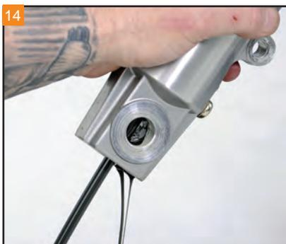
14 Allow the old fork oil to drain into a suitable container.
