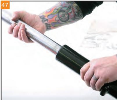
Slide the fork leg assembly into the fork slider.
