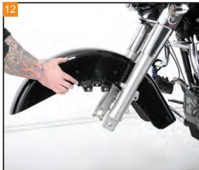
12 Remove the fender from in between the fork legs from the front.
