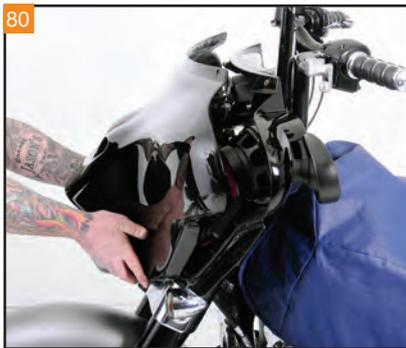
80 Bring the outer fairing into position, plugging in the headlight wiring connector before placing the outer fairing on the bike.
