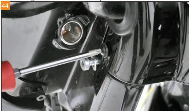
44 With a T27 Torx, remove the two bolts per side holding the lower inner fairing.
