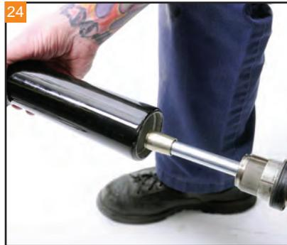
24 After installing the bottom cup, install the fork leg into the slider.
