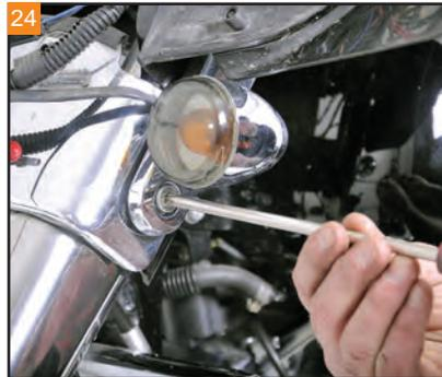
With a T40 Torx, remove the two bolts per side holding the turn signals in place.
