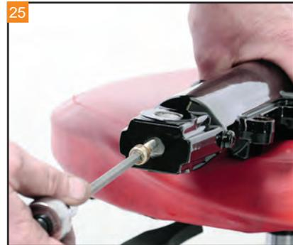
25 Use a long 6mm Allen to tighten the damper bolt from the bottom of the fork slider.
