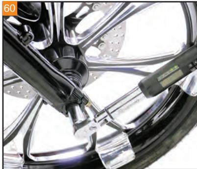
60 Final torque of the Klock Werks' Axle is 40-45 foot/lbs.
