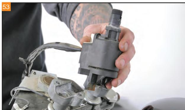
Lift the ignition switch assembly off the top triple trees.
