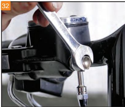
Loosen the banjo bolt at the front master cylinder to remove the brake line. Have a small drain pan ready to catch any brake fluid when removing the bolt.
