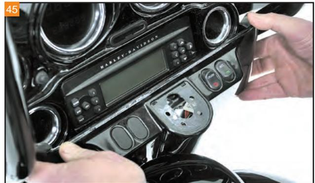
45 Lift the lower inner fairing up and off the ignition post to access the wiring underneath.
