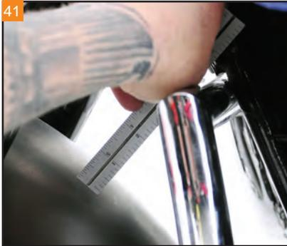
Use the scale to measure the distance between the top of the fender and the first point of potential contact.
