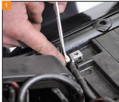
1 Remove the seat. Use a 10mm wrench to disconnect the ground wire to the negative terminal of the battery.
