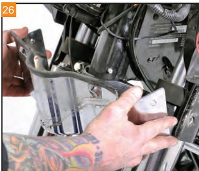
With both turn signals removed, the lower outer fairing skirt can be removed from the front end.
