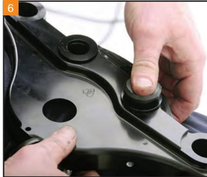
Install the riser bushings with center spacers.
