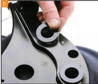
Place the bushing spacers on the upper triple tree.
