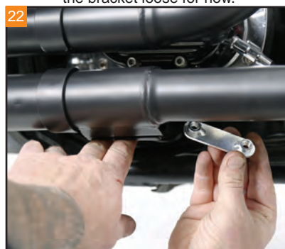
Start the included hardware that holds the exhaust to the transmission side bracket. Do not final tighten: leave the bolts loose for now.
