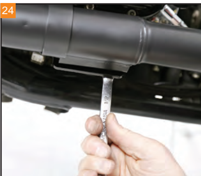
With a 1/2" wrench and 1/4" Allen, final tighten the bracket and mounting hardware.
