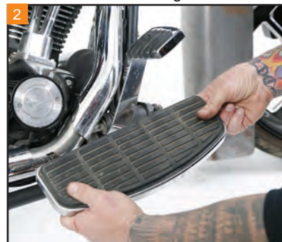
Remove the right side floorboard from the mounting brackets.
