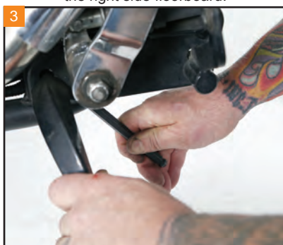
With a 3/8" Allen wrench, loosen the bolt holding the right rear floorboard-mounting bracket to the frame. Rotate the bracket down and out of the way.
