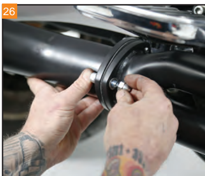
Apply blue thread locker to the bolts. Start the three end nuts with washers.
