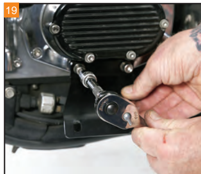
Install the new Covington's bracket using the stock hardware. Apply blue thread locker to the bolts, but leave the bracket loose for now.
