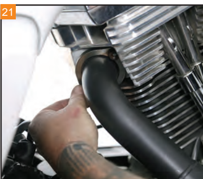
Start the flange nuts on the studs of the heads by hand. Leave the nuts loose for now.
