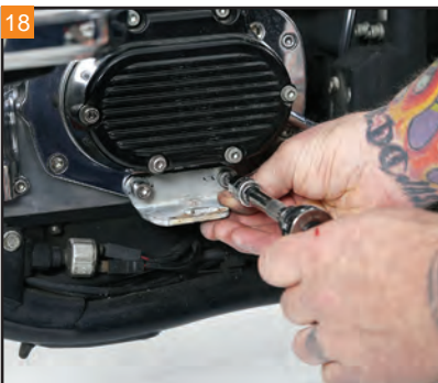
Use a 1/4" Allen to remove the stock bracket from the trap door of the transmission.
