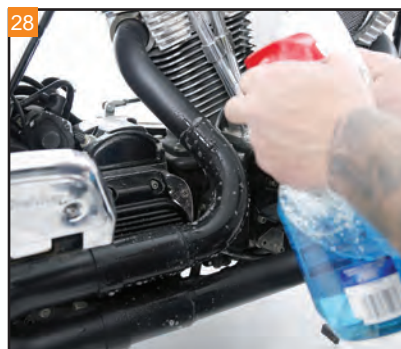
Prior to installing the heat shields, clean the exhaust with glass cleaner and shop towels to remove all grease and fingerprints.
