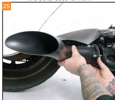
Using the included gasket and hardware, connect the Destroyer Exhaust end piece to the head pipes.
