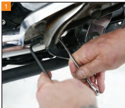
Use a 3/16" Allen and 7/16" wrench to remove the hardware holding the right side floorboard.
