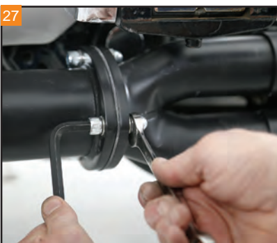
Uniformly tighten the three bolts with a 5/16" Allen and a 9/16" wrench. The outer most bolt may have to be removed in order to install the collector heat shield.
